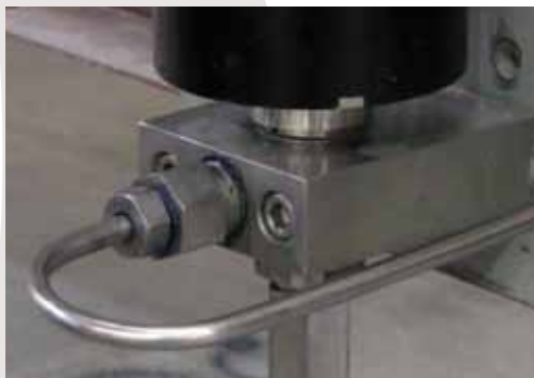
1/4" Thimble Filter threaded directly into the cutting head.
