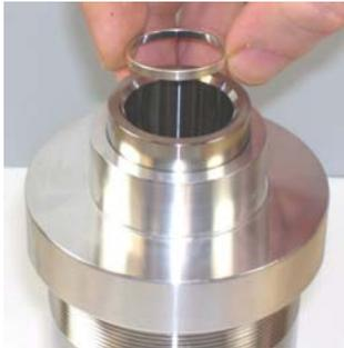
10. Place the Hoop with the sharp (tapered) end down into the installation sleeve.
