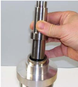
9. Use the blunt (non-stepped) end of the installation tool to hand press the seal the rest of the way into the cylinder.
