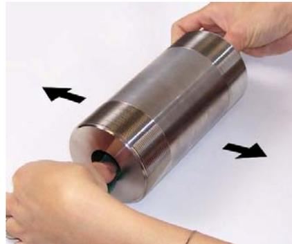
5. To refinish the ID cylinder bore, place the cylinder on a table and with a piece of **180** grit abrasive paper in *each* end and roll the cylinder back and forth to remove any blemishes. Repeat this process with **Scotch Brite** to polish the surface. Clean the cylinder thoroughly after polishing.
