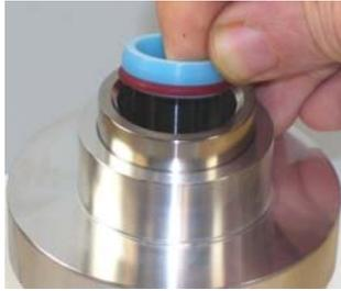
8. Lubricate the ID of the Sleeve with grease and load the seal with the o-ring side down into the sleeve. Keep the seal square while inserting it into the sleeve with your fingers.
